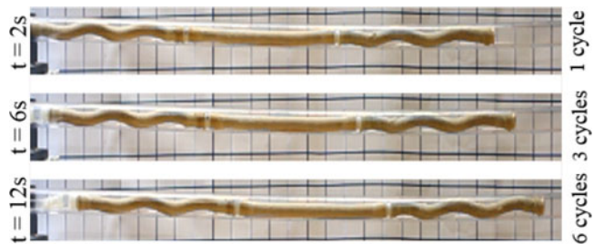
Fig. 14. Soft robot locomotion through a cannula at different time steps. The images were captured at full anchoring, Event D (See Figs. 2(a) and 13).
