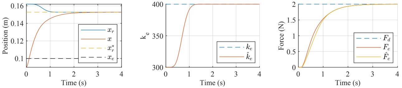
Fig. 3. Position tracking depicting convergence of  $x$  to both  $x_r$  and  $x_r^*$  (left), estimation of environment stiffness with  $\hat{k}_e$  converging to the true value  $k_e$  (center), and force tracking of the environment force,  $F_e$ , converging to the desired force,  $F_d$  (right) for simulation trial B
