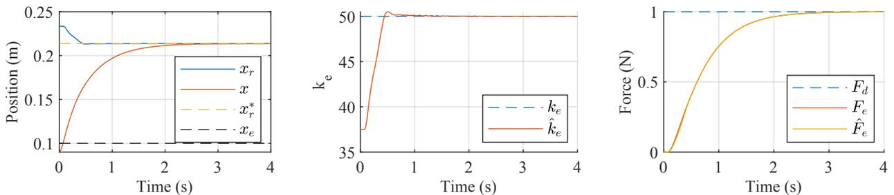
Fig. 2. Position tracking depicting convergence of  $x$  to both  $x_r$  and  $x_r^*$  (left), estimation of environment stiffness with  $\hat{k}_e$  converging to the true value  $k_e$  (center), and force tracking of the environment force,  $F_e$ , converging to the desired force,  $F_d$  (right) for simulation trial A
