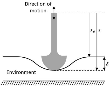
Fig. 1. Schematic of 1-DOF interaction with environment
