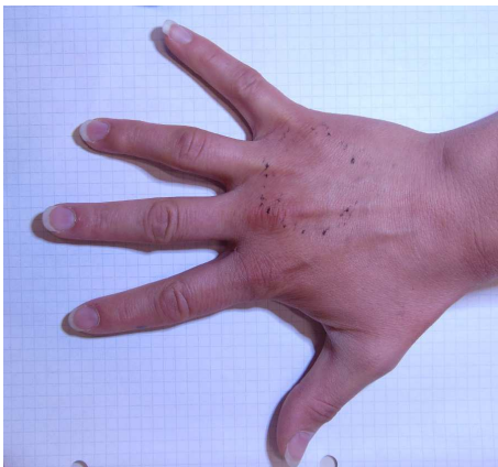
Figure 16: Printing of a 4cm diameter dotted circle on a human hand
