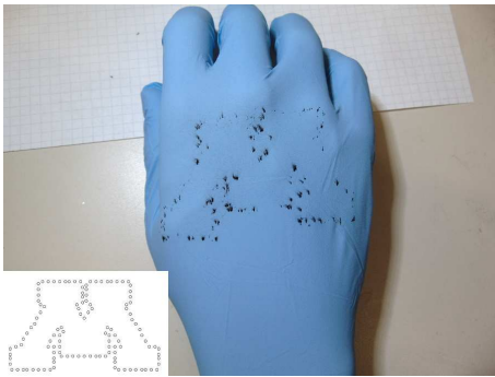
Figure 15: Printing a shape outline (see inert) under simulated hand motion
