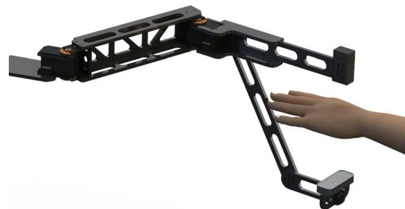
**Fig. 2 Solid model rendering of kinematically optimized two-link robot design**
