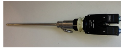
Fig. 2. The da Vinci camera unit and Endoscope.
