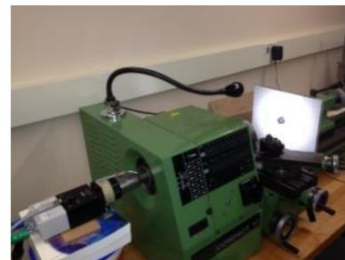
Fig. 2 Calibration routine using lathe
