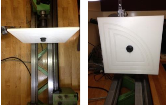
Fig. 3 Reference trajectory in lathe
